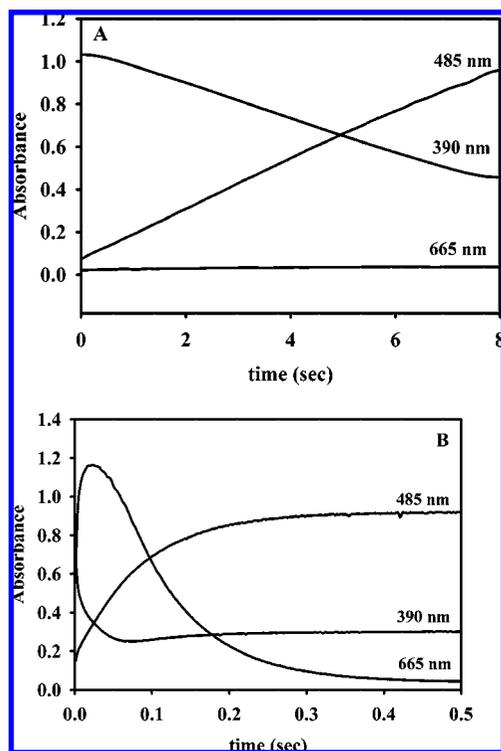
**Figure 4.** Stopped-flow traces of the reaction of Co(II)-containing L1 analogues with nitrocefin. 50  $\mu$ M 1Co- (A) and ZnCo-L1 (B) analogues were reacted with 50  $\mu$ M nitrocefin at 4  $^{\circ}$ C. The absorbance at 485 nm is due to the product, the absorbance at 390 nm is due to the substrate, and the absorbance at 665 nm is due to the intermediate.
