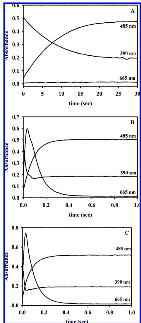
**Figure 7.** Stopped-flow traces of Fe-containing L1 analogues reacted with nitrocefim; 50  $\mu\text{M}$  1Fe-L1 (A), ZnFe-L1 (made by adding Fe(II) to 1Zn-L1) (B), and ZnFe-L1 (made by adding Zn(II) to 1Fe-L1) (C) were reacted with 50  $\mu\text{M}$  nitrocefim at 4 °C. The absorbance at 485 nm is due to the product, the absorbance at 390 nm is due to the substrate, and the absorbance at 665 nm is due to the intermediate.
