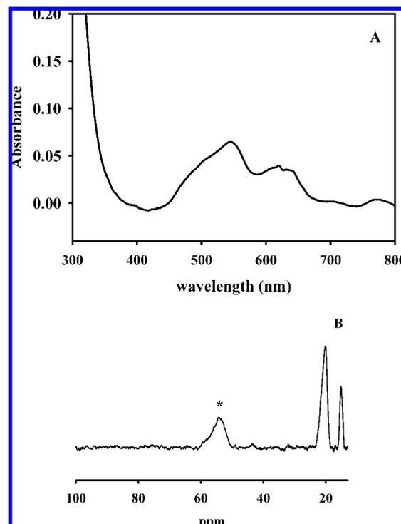
**Figure 1.** UV-vis and NMR spectra of 1Co-L1. (A) UV-vis difference spectrum of 1Co-L1 prepared using biological incorporation method. The enzyme concentration was  $550 \mu\text{M}$ , and the buffer was 50 mM Hepes, pH 7.0. (B) <sup>1</sup>H NMR spectrum of  $550 \mu\text{M}$  1Co-L1. The asterisk signifies the peak that is solvent-exchangeable.
