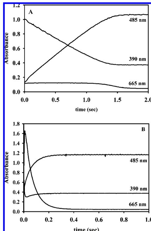
**Figure 3.** Stopped-flow traces of the reaction of Zn(II)-containing L1 analogues and nitrocefin. Stopped-flow traces of 50  $\mu\text{M}$  1Zn-L1 (A) and ZnZn-L1 (B) analogues when reacted with 50  $\mu\text{M}$  nitrocefin at 4  $^\circ\text{C}$ . The absorbance at 485 nm is due to the product, the absorbance at 390 nm is due to the substrate, and the absorbance at 665 nm is due to the intermediate.<sup>54</sup>
